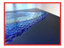
The spot layer is at least 20-30 micron (0,2-0,3 mm) in thickness. The elevated structure of the effect can be
